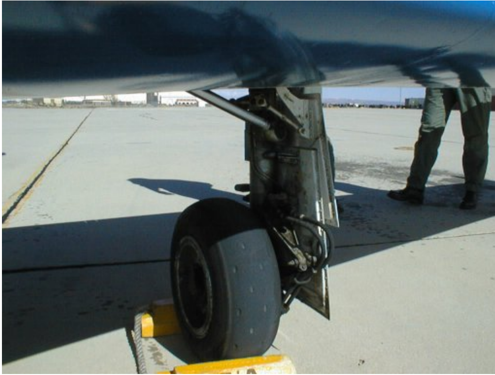
The main landing gear retracts inward into the wing.
